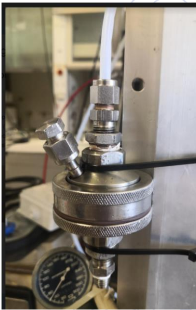
Figure: System to hold the filter
